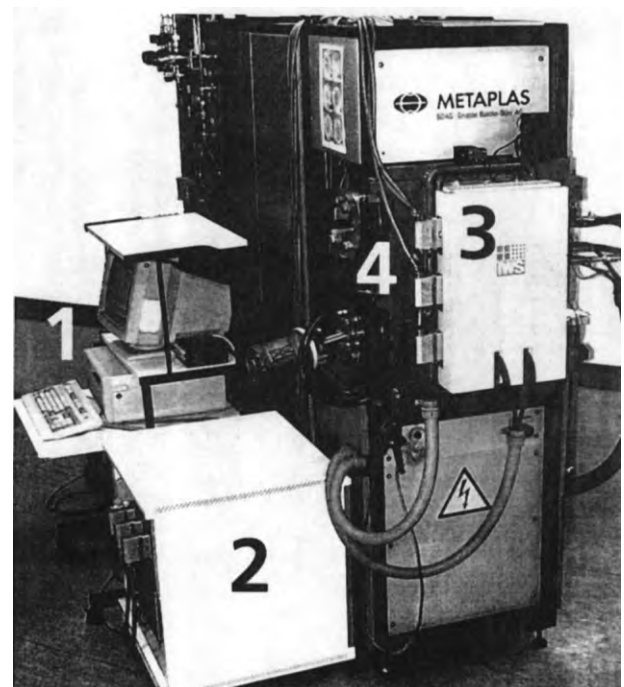
Fig. 3. ProArc-system assembled to a vacuum-arc coating device: 1, computer; 2, multi-channel power source; 3, coil array with 24 coils; 4, coating chamber.
