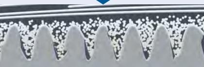
During cooling, the polymer solidifies and thus enables a firm joint between metal and plastic.
