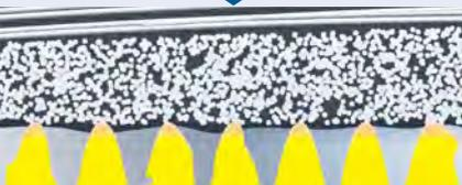
The joining partners are aligned and pressed together. The heat induced into the metal melts the plastic and causes it to infiltrate the metal structure.
