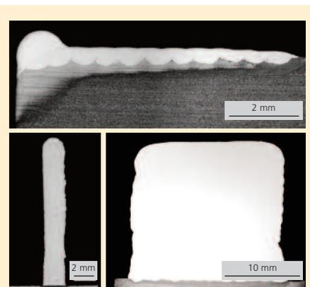
*Cross sections of representative examples: cladding on edges, thin wall structures and generation of volume parts*
