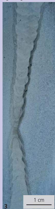
Weld (microsection) after laser welding using the 10 kW diode laser
