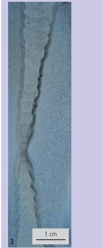
Weld (microsection) after laser welding using the 10 kW diode laser
