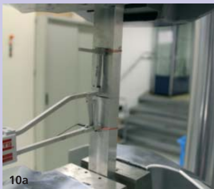
Characterization of the samples that have been Laser-MPNG welded in the tensile test (10a), failure behavior of apparent material sample (10b left) and a welding seam obtained by Laser-MPNG welding (10b right)
