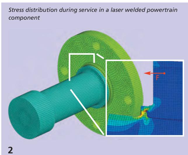
Stress distribution during service in a laser welded powertrain component
