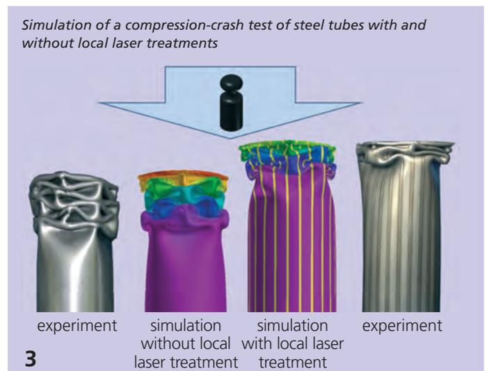
Simulation of a compression-crash test of steel tubes with and without local laser treatments
