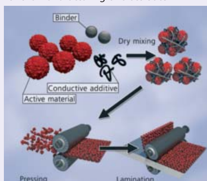
Scheme of the solvent-free dry film process for the manufacturing of electrodes
