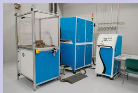
Fig. 5: Commercially available magnetic pulse welding machine
