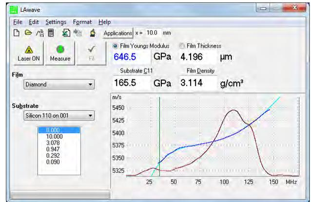
Figure 5: Measured dispersion curve (dark blue) and fitted theoretical dispersion curve (light blue) for a silicon substrate with a diamond film. The pulse amplitude is shown as a brown line. The elastic moduli of film and substrate were calculated by fitting.
