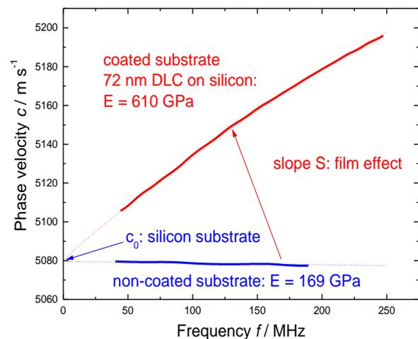
Figure 1: Effect of a 72 nm thick DLC film on the phase velocity  $c$  of the surface acoustic wave versus the frequency  $f$ . Solid lines represent measured data, dashed lines the fitted theoretical model.
