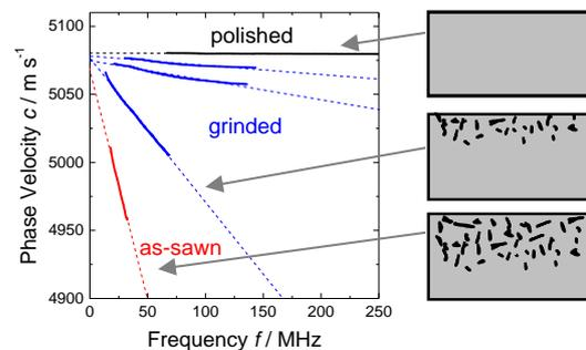
Figure 9: Dispersion curves measured on silicon wafer surfaces in the as-sawn, grinded, and polished state.
