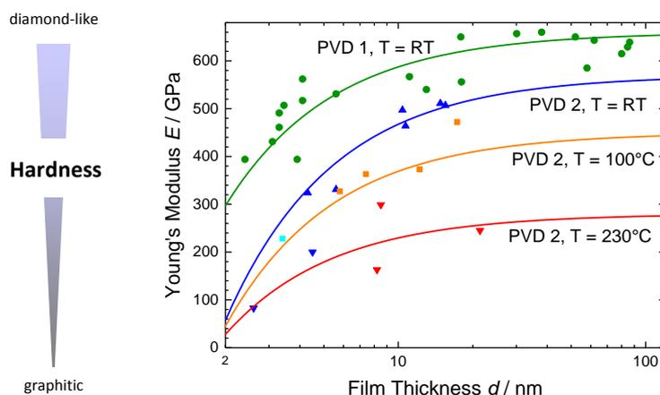
Figure 7: Young's modulus of hydrogen-free DLC coatings in dependence of coating thickness, showing the influence of deposition temperatures and different PVD technologies.
