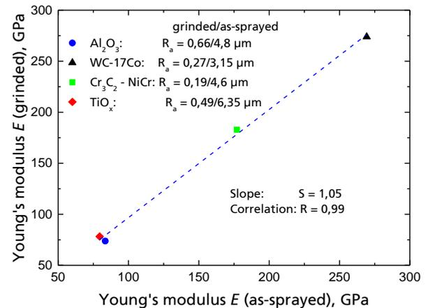
Figure 10: Comparison of Young's modulus of different thermal-sprayed coatings measured with LAwave on the rough, as-sprayed surface and the grinded surface
