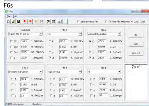
Figure 6: Screenshot of program windows for fitting single layer (F5s) and multi-layer (F6s) systems. The graphic window displays both the measured dispersion curve and the fitted theoretical model.
