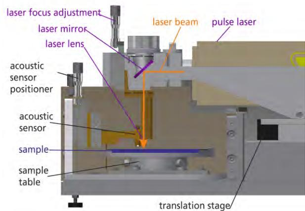
Figure 3: Cross section of the LAwave device, showing laser, optical, sample, and sensor components
