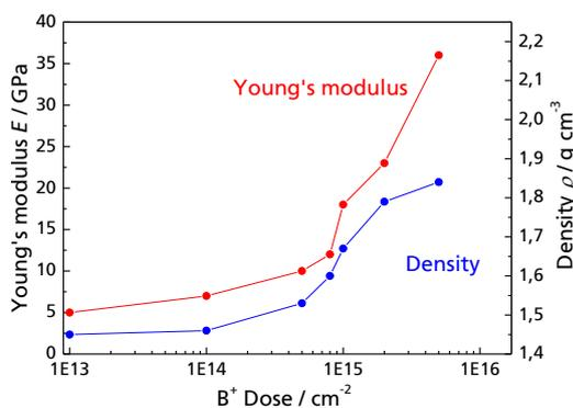
Figure 8: Young's modulus and density of polymeric sensor films versus the B<sup>+</sup>-ion implantation dose. Fitting the dispersion curve yielded both material parameters from one measurement.
