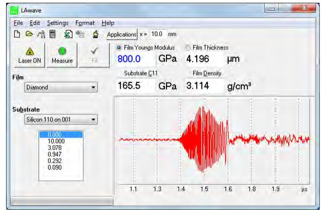
Figure 4: Laser-acoustic signal detected on a silicon substrate with a diamond film
