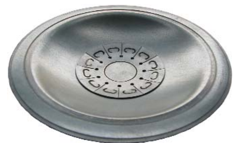
Fig. 1: Formed model part with optimized patch and welding seam contour
