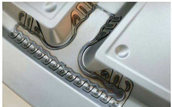
Fig. 2: Demonstrator: engine hood with edge relaxed patch
