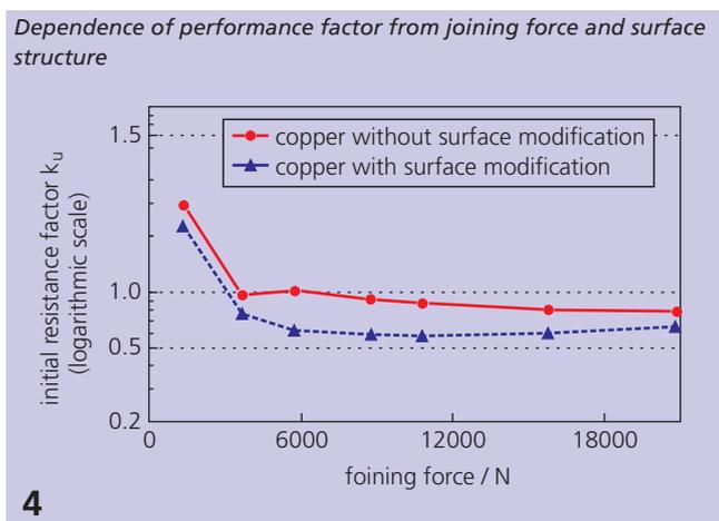
The quality of a connection is evaluated by the performance factor  $k_u$ , which allows a comparable representation of different materials and contact cross sections. This factor is the ratio of the resistance of the connection  $R_V$  measured over a length  $l_V$  to the resistance  $R_L$  of the homogenous conductor material with the same geometry and length  $l_L$ . If  $k_u = 1$  then the power loss and heating over the connector is equal to the power loss over the regular metal conductor.
