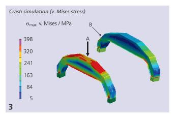
pure elastic material behavior. The calculated stress distributions and part deformations were analyzed and the component design was iteratively improved. A boundary condition during this optimization was to minimize the component mass.
