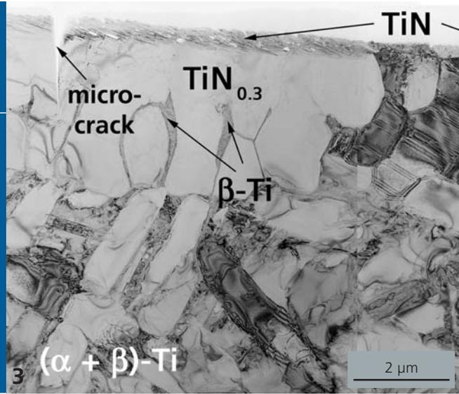
by reducing the nitrogen content of the processing gas and additionally if the thin top layers are removed by grinding or shot peening.
