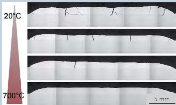
Crack prevention due to localized process simultaneous additional heating: cross section of an area coating from Stellite 20, 62 HRC
