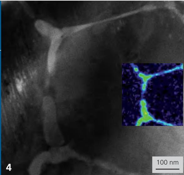
Another research topic at Fraunhofer IWS is the development of reactive multilayer coatings (RMC), which are applied in low heat impact joining processes for various material combinations (see pages 86 / 87). An important aspect of this development is to avoid diffusion within the coating stack during the fabrication. TEM analysis demonstrated that specific barrier coatings help to avoid this undesired diffusion effect (Fig. 2).
