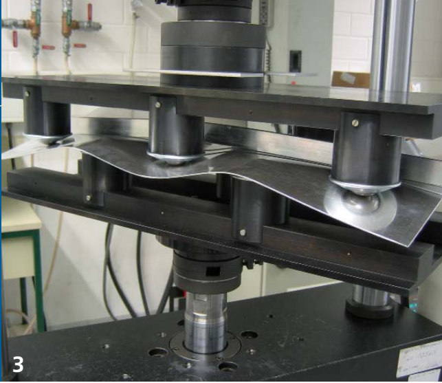
Maximal bending load in a ten-point bending experiment for various stringer geometries
