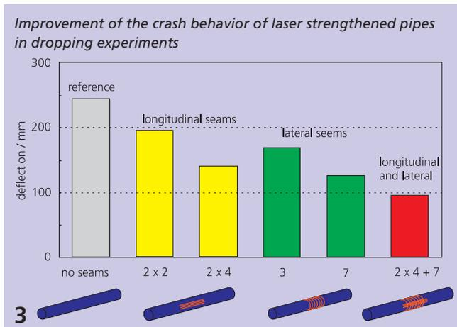
Additional dropping experiments with laser strengthened pipes also showed a clearly reduced deflection (Fig. 3).
