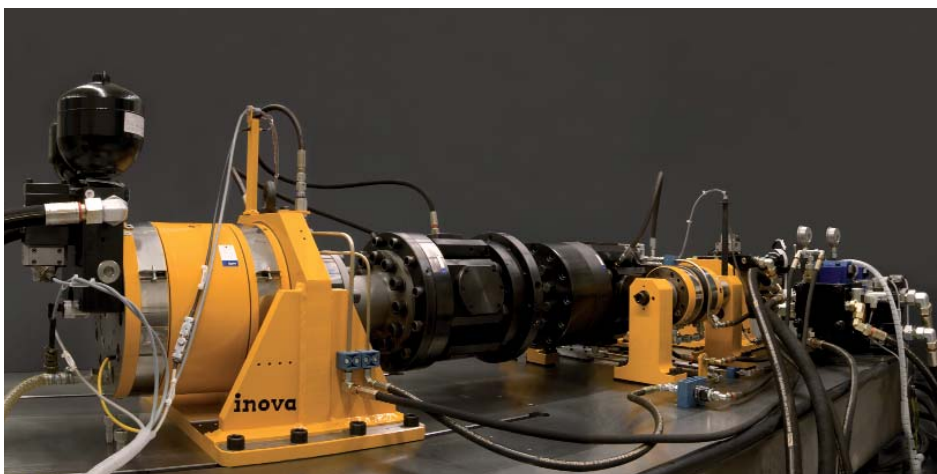
Fig. 2: Torsion-axial testing system
