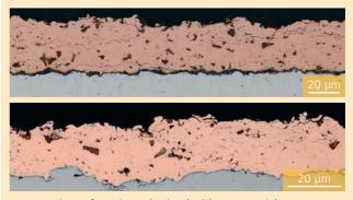
A comparison of coatings obtained with commercial copper powder including alumina particles, fabricated without (top) and with (bottom) laser support. Positioned such that it runs ahead of the spraying particle beam, the laser spot improves bonding to the substrate.
