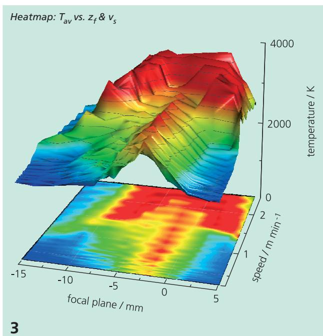
The melt pool characteristics depend on many factors, with various effects. The melt pool characteristics are strongly influenced by the sheet metal thickness, the laser power, and the resultant cutting clearance geometry.
