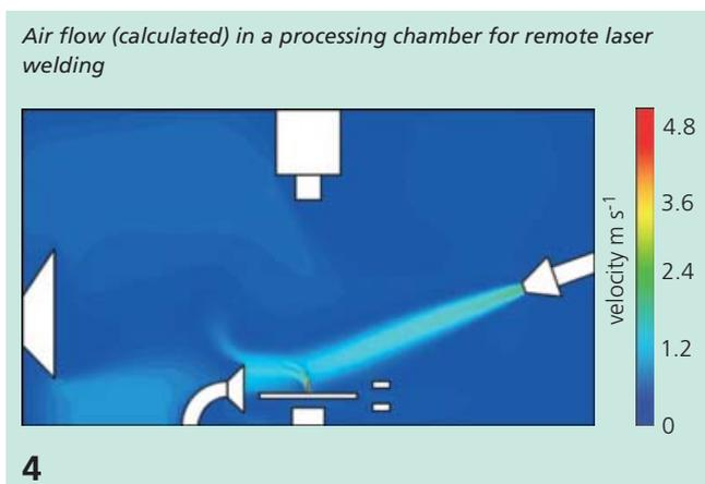
The purpose of the project is to evaluate concepts of optimized air flow guidance, which, on the one hand, eliminate disturbing welding vapors in the laser beam path. On the other hand, they also guide the process emissions intentionally into the designated exhaust units to minimize the contamination both of workpieces and optical components. Flow characteristics of individual components were found to be a specific challenge and have usually to be analyzed separately in submodels.
