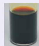
E2: IWS electrolyte system, low lithium polysulfide solubility
