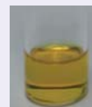
E2: IWS electrolyte system, low lithium polysulfide solubility
