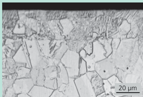
Heat affected zone at the cutting edge
