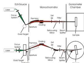
Photograph of the EUV reflectometer and schematic representation of the beam path (front and top view).
