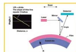
The laser scanning method is used to measure the wafer curvature. With the commercial tool FLX-2320 (KLA-Tencor) sample annealing up to temperatures of 500 °C and in-situ stress measurements are possible.
