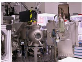
Photograph of the thin film deposition machine "UHV cluster tool" combining two deposition chambers, the handling system, one sample magazine and the load-lock. In both deposition chambers, MSD and PLD, up to four materials can be used in the multilayer period. The typical substrate size is  $\varnothing = 150\text{ mm}$ , the maximum size can be up to  $\varnothing = 250\text{ mm}$ .
