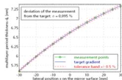
Typical precision of layer thickness gradients obtained using transmission masks. For one-dimensional gradients deposited with special velocity profiles of the substrate motion the precision is typically by a factor of 2 better.
