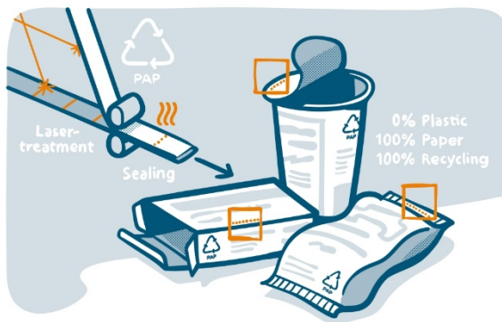
Fig. 1 Process for sealing a laser-modified paper web without additives
