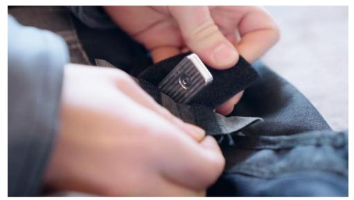
Flowable materials integrated into firefighters' clothing absorb PAH like a sponge, and electrical sensors record contamination in the field. © Veritas Medien GmbH/BLAULICHTKANAL
