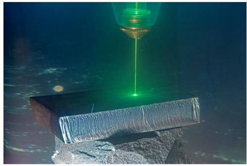
A particularly short-wavelength green laser, whose cutting capability is also given in water, is used to cut steel and metals in the sea. Fraunhofer IWS has researched and developed a solution that already works in the lab. © Fraunhofer IWS PRESS RELEASE No. 10 | 2023 August 30, 2023 || Page 3 | 3
