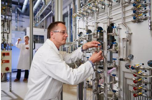
The researchers at Fraunhofer IWS use a multi-adsorption system to investigate the adsorption behavior of competing gases to find suitable filter substances.
