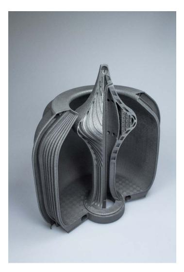
A design demonstrator for an additively manufactured aerospike nozzle © Fraunhofer IWS Dresden
