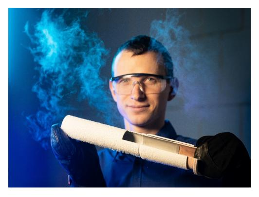
Magnetic pulse welding is able to create substance-to-substance joints between dissimilar materials like copper, aluminum and steel. The method fulfills the tightness requirements even at very low temperatures, in systems for storing and distributing liquid hydrogen for example. © ronaldbonss.com
