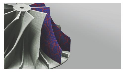
For the first time, scientists at Fraunhofer IWS printed 3D high-entropy demonstrator structures made of the Cantor alloy "CrMnFeCoNi" using the Fused Filament Fabrication (FFF) process. On the surface, the illustration shows an example of a particularly high-strength microstructure consisting of two phases as a planned further alloy system development. © Fraunhofer IWS Dresden
