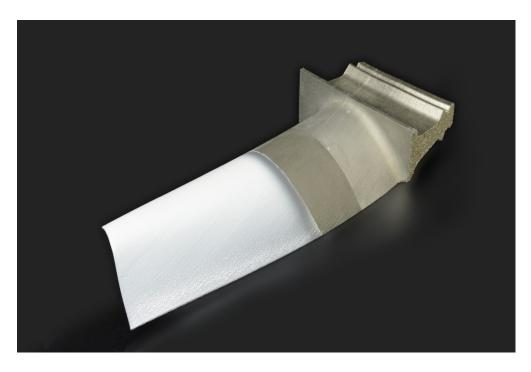
Turbine blade with a thin ceramic coating of yttrium-stabilized zirconium oxide (YSZ): such a thermal barrier coating allows a higher operating temperature in the turbine, which improves the fuel yield.
