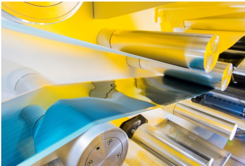
Roll-to roll: innovative and efficient procedure for the fabrication of solar foils. © Heliatek / Baldauf & Baldauf
