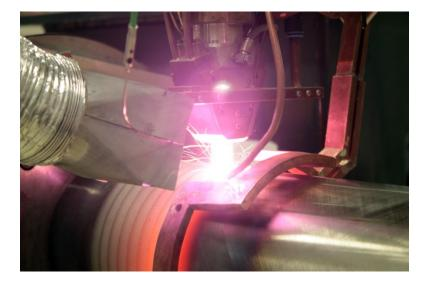
While turning a Laser is guided along the processed cylinder rod with an even forward feed. © Fraunhofer IWS Dresden
