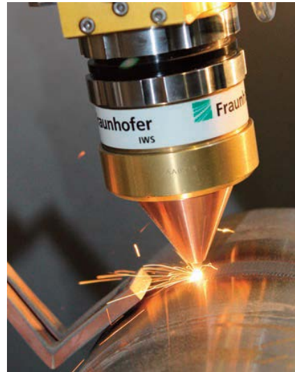
Laser buildup welding with a COAX laser processing head © Fraunhofer IWS Dresden
