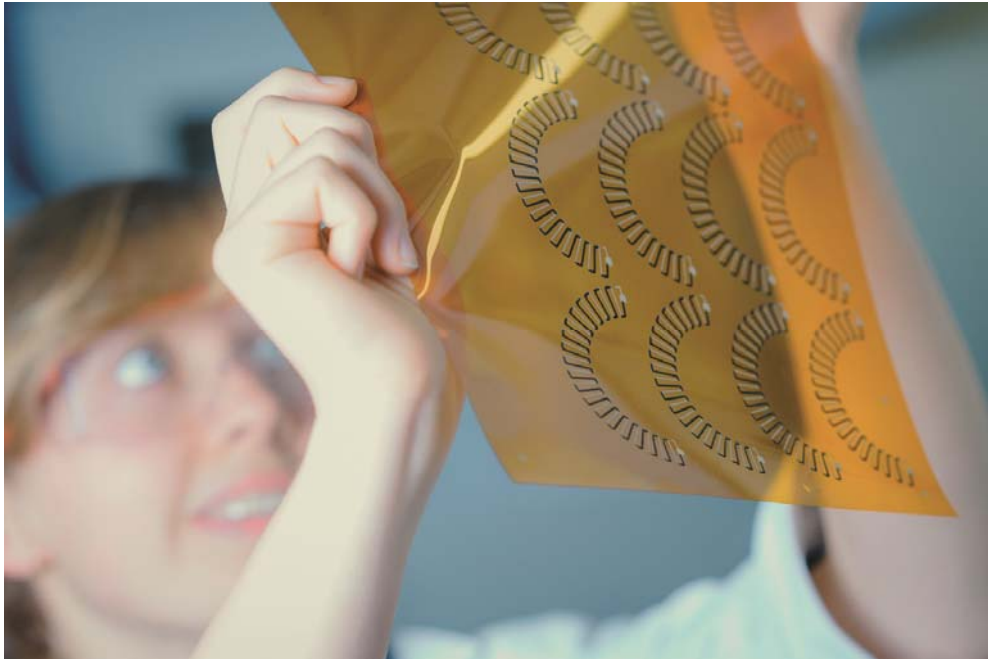
Printed thermoelectric module with flexible geometry © Fraunhofer IWS Dresden
