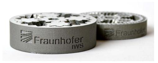
A planetary gear, created in one process step (without joining) © Fraunhofer IWS Dresden
