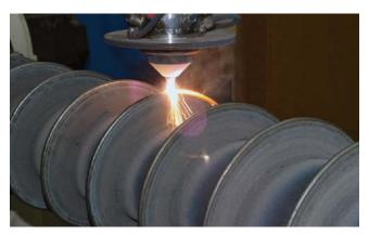
An additive manufacturing process with a laser beam onto an extruder screw made from stainless
