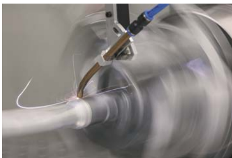
Laser beam cutting of die-cast aluminum components © Finow Automotive GmbH / Steffen Herre
