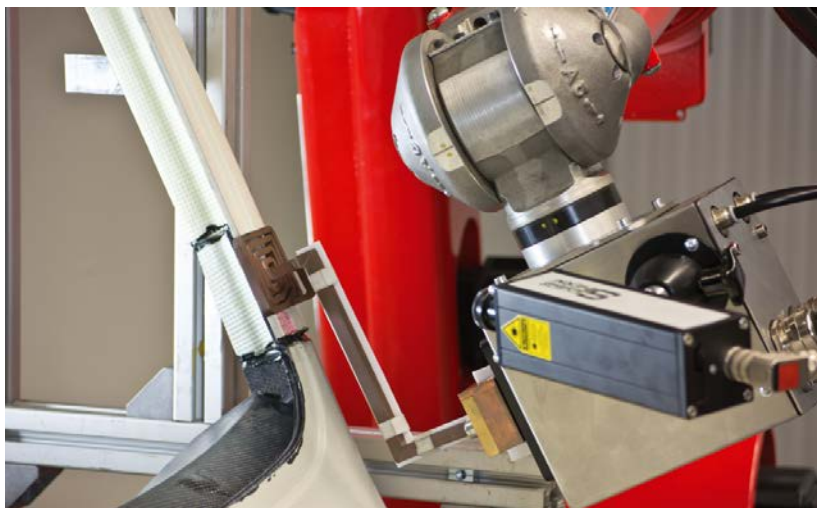
Pyrometer-controlled inductively accelerated adhesive hardening with industrial robot © Fraunhofer IWS Dresden
