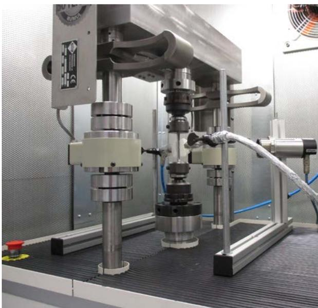
Notched steel sample during tensile test
