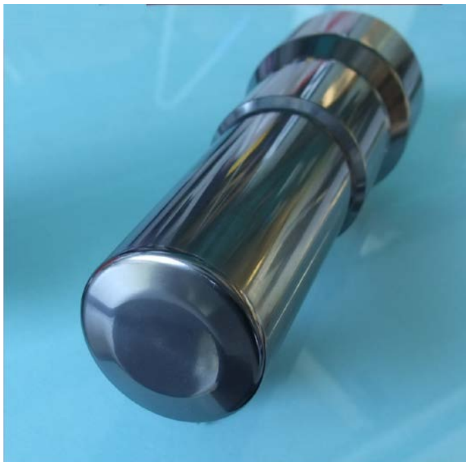
Forming tool, coated with 10 \mu\text{m} AlCrSiN/TiN- nano-composite layer © Fraunhofer IWS Dresden
