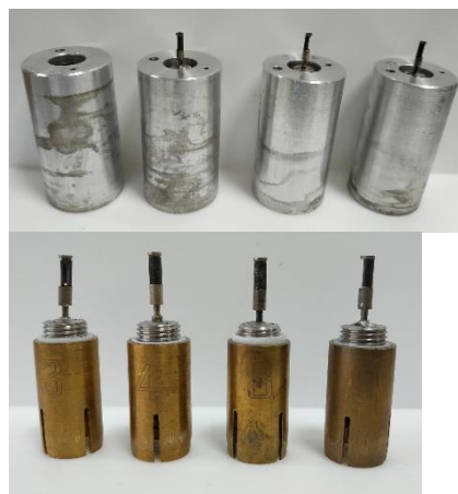
Micro cells with stainless steel blocking electrodes
