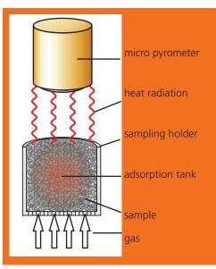
The degree of temperature rise and the temperature profile are the indicators for the adsorption capacity. The rapid test device infraSORB is able to characterize simultaneously and within only few minutes up to 12 samples regarding their porosity.
