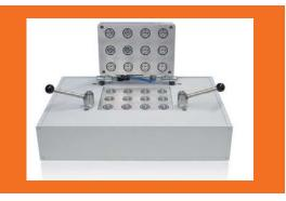
The test sample is thereby exposed to a gas flow which contains the gas to be adsorbed. If adsorption takes place on the material, adsorption heat will be released. This heat is continuously measured by using a contactless optical temperature sensor.
