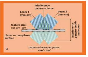
This method involves the modulation of the laser beam intensity by generating interference patterns, see Figure (a). In this way, the regions corresponding to the interference maxima positions can be locally ablated, molten or modified. Depending on the number of laser beams interfering on the substrate surface, a wide range of 2D and 3D micro- and sub-micrometer periodic
