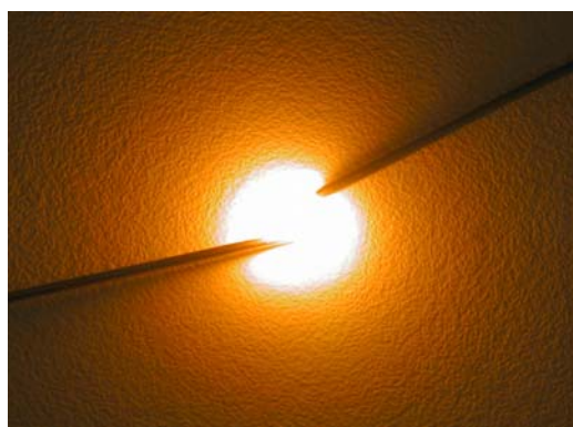
Figure 2: Ignition of a reactive nanometer multilayer foil by an electrical spark
