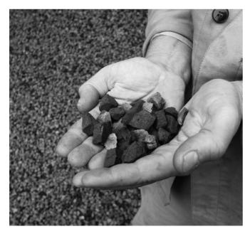
Processed material recovered from slag. (© Fraunhofer UMSICHT) | Picture in color and printing quality: www. fraunhofer.de/press
