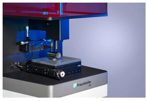
In the pictured configuration the LAwave measuring system allows the fast and non-destructive characterization of small and medium-sized components.
